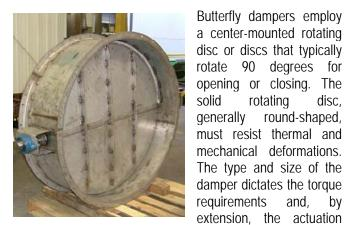
requirements (e.g., beyond a certain torque, pneumatic actuators become less desirable than hydraulic dampers due to their size).
