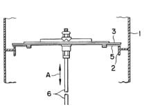
pneumatic actuator. When the flat plate is in the closed position, it provides a gas seal by pressing against a seat, shaped like a short cylinder. Gas attempting to pass through the cylinder is blocked by the poppet plate. When the damper is open, there is a one- to two-foot gap between the flat plate and the cylinder opening. Poppet dampers are used for on-off control only; they are not appropriate for modulating applications.
