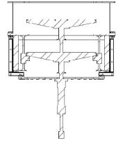
Poppet dampers of this type are driven with pneumatic or hydraulic cylinder actuators for high-cycle service and
