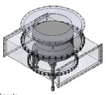
Poppet dampers with three-way and four-way configurations
