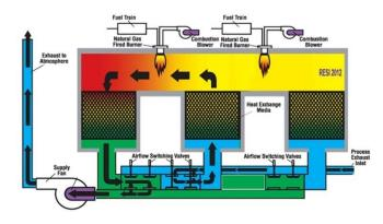
The major components of an RTO system consists of heat exchange canisters, combustion chamber, and multiple valves or dampers. The RTO system consists of multiple heat recovery chambers. The air is cycled through an inlet chamber for preheating and an outlet chamber for reheating the heat exchanger bed before exiting. Before chambers switch from inlet to outlet flow, they are purged of any residual VOC laden gas. This purging ensures minimal VOC spikes and maximizes destruction efficiency.
